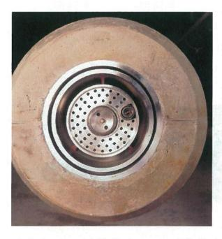
A constant momentum can only be maintained by adjusting axial air as well as swirl air.
