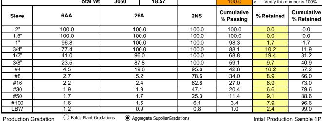
Coarseness Factor: 62 **Workability Factor:** 34 JMF Zone 75. 39 Workability Factor (%) ■ 60, 36 IPS Production Gradation 52, 34 Operating Zone 75, 28 Boundary 45 50 Coarseness Factor (%) $^{70}$ 75 80 ActionLimits Boundary = - - - - -
